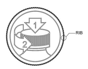
DETAIL RIB SCALE 6 : 1 (88) EQUISPACED RIBS
