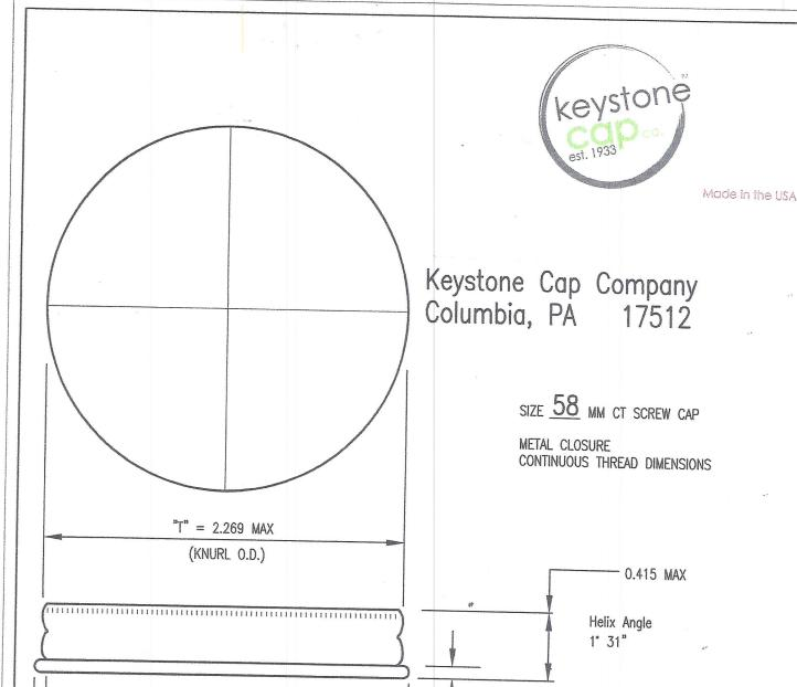
The Max & Min. inside diameter of the thread are determined by round Max & Min plug gauges. The closure should permit entry of the min guage and no entry with a slight drag on the max gauge.
